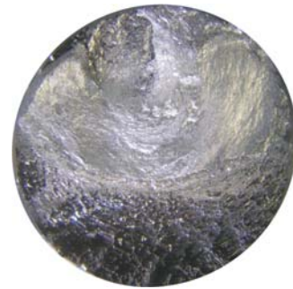
Fig. 8. Crosssection of fatigue scrap
